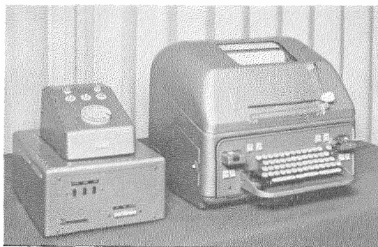
Figure 1—Subscriber station with laboratory model of GH 111 error-detection set.
